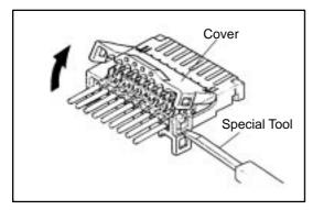
(2) w/ Cover : Open Connector Cover Using a special tool, release the lock and open the cover.
