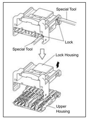
Type L (0.64 of Insulation Displacement Connector (IDC) Type)
