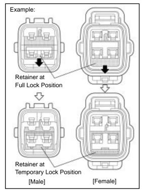
(1) Insert the tool straight into the access hole of terminal retainer as shown.
