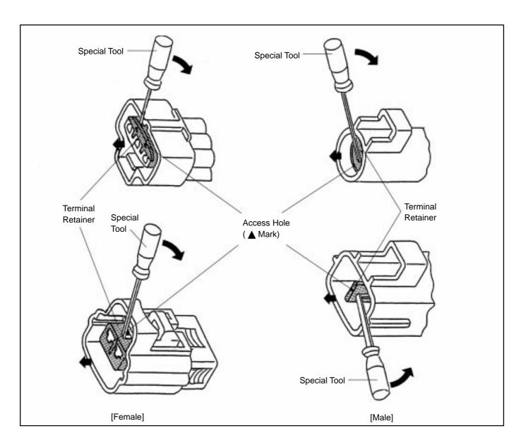
(1) Insert the special tool into the terminal retainer access hole (▲ Mark) and pull the terminal retainer up to the temporary lock position.
