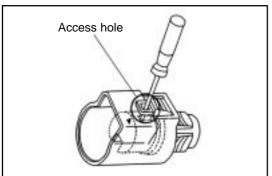
HINT: In some cases insert the special tool from the access hole on the flank of the housing.
