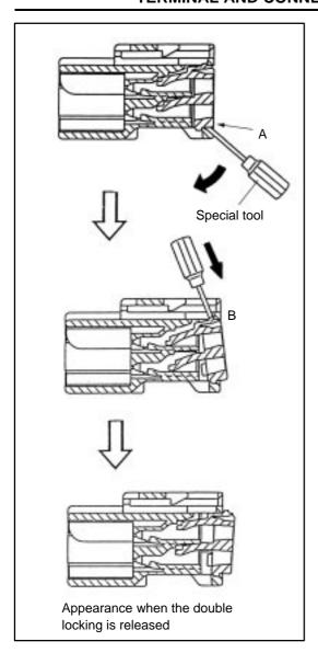
(1) Insert the special tool into the service hole and move it to the direction of the arrow to release the lock on the side A.
