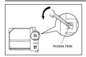
(1) Press the special tool at a 45° angle into the locking lug access hole as shown.
