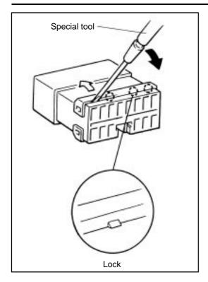
(2) Inset the special tool into the chink between the retainer and the terminal itself. Then pry it to the direction of the arrow shown in the illustration and push the retainer up to release the lock.
