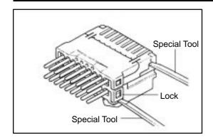
Type J (For Insulation Displacement Connector)
