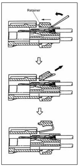
(2) Move the special tool to the direction of the arrow and release the lock.
