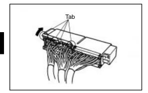
(2) Remove the special tool and open the double locking device
